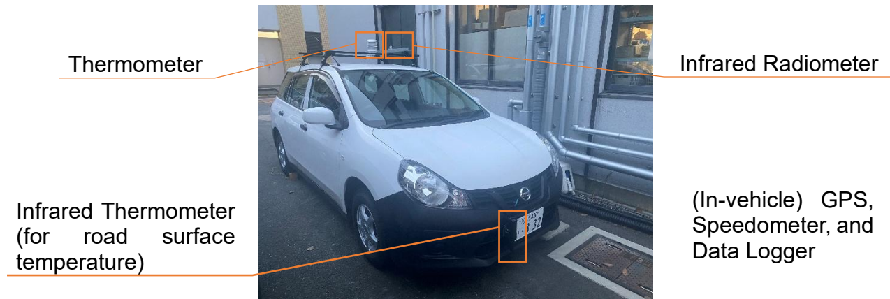
Figure-2 Sensor Mounting Position
